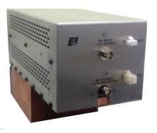
The M-0240L-T Amplifier Module is a rugged source of RF power, useful for ultrasonics, laser modulation, RFI/EMI, plasma equipment and general laboratory applications. This module is designed to be integrated in to a system. It requires a DC voltage input and forced air cooling. The M-0240L-T represents E&I's commitment to providing RF power amplifiers of the highest quality, durability and ruggedness.
