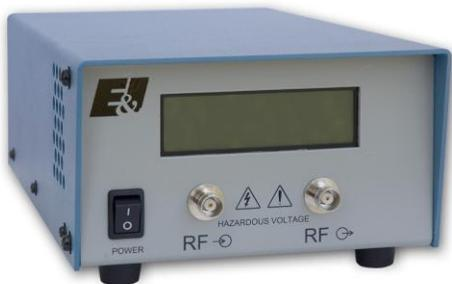
The PI-30 RF power indicator is used to measure the RF level of signal sources in the 1 to 30 MHz range. This portable unit is self-contained with an easy to read LCD display, no tuning or any other form of adjustment is required.
