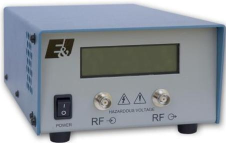
The PI-10 RF power indicator is used to measure the RF level of signal sources in the 100 KHz to 10 MHz range. This portable unit is self-contained with an easy to read LCD display, no tuning or any other form of adjustment is required.
